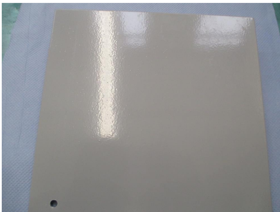
Fig 2: Photograph showing the condition of the Grey Powdercoat Plate Sample after 216 hours Salt Spray Test
